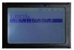
b) In accordance with actual situation, select the corresponding ecu, press OK button, will display the ECU information
