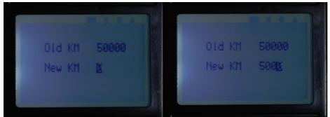
Note: Some instruments, need to manually enter the old mileage, and some instruments can be directly read the mileage. If the mileage can not automatically read the meter, enter the current mileage meter, for example, the A6L Marelli instrument which is CAN interface, need to manually enter the old mileage.
